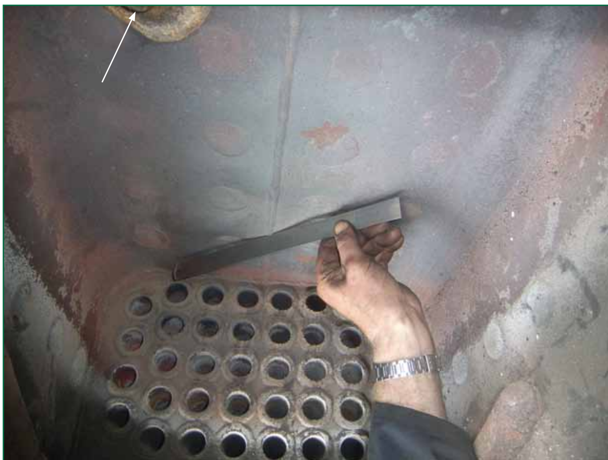
Figure 7: Interior of firebox showing scorch marks and quilting of the crown (location of fusible plug arrowed)
