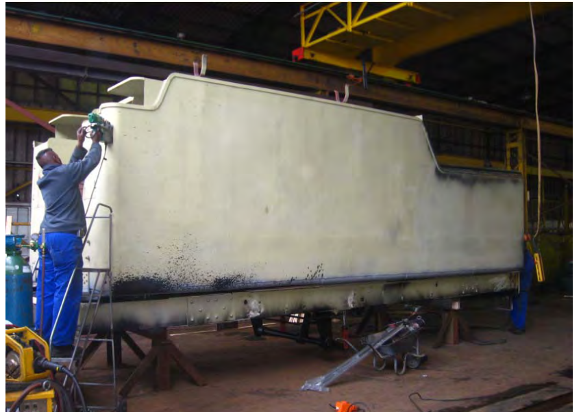
The tender seen under restoration is no. 2737 and has been given a complete overhaul in preparation for use with Class 3BR 1486 – first trip scheduled for Sunday, 28 November. (Marc Bouchier).
