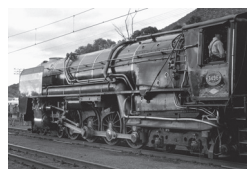
Condenser No. 3486 handling the 30th anniversary Blue Train in 1969. The locomotive is in final condition, train Hardy safety valves exhausting to the steam pipe. Notice water separator in front of the firebox, raised lagging cover over the cross and radial flexible stays and L.H. blowdown buffer drum. Photo L. Pinnis.
