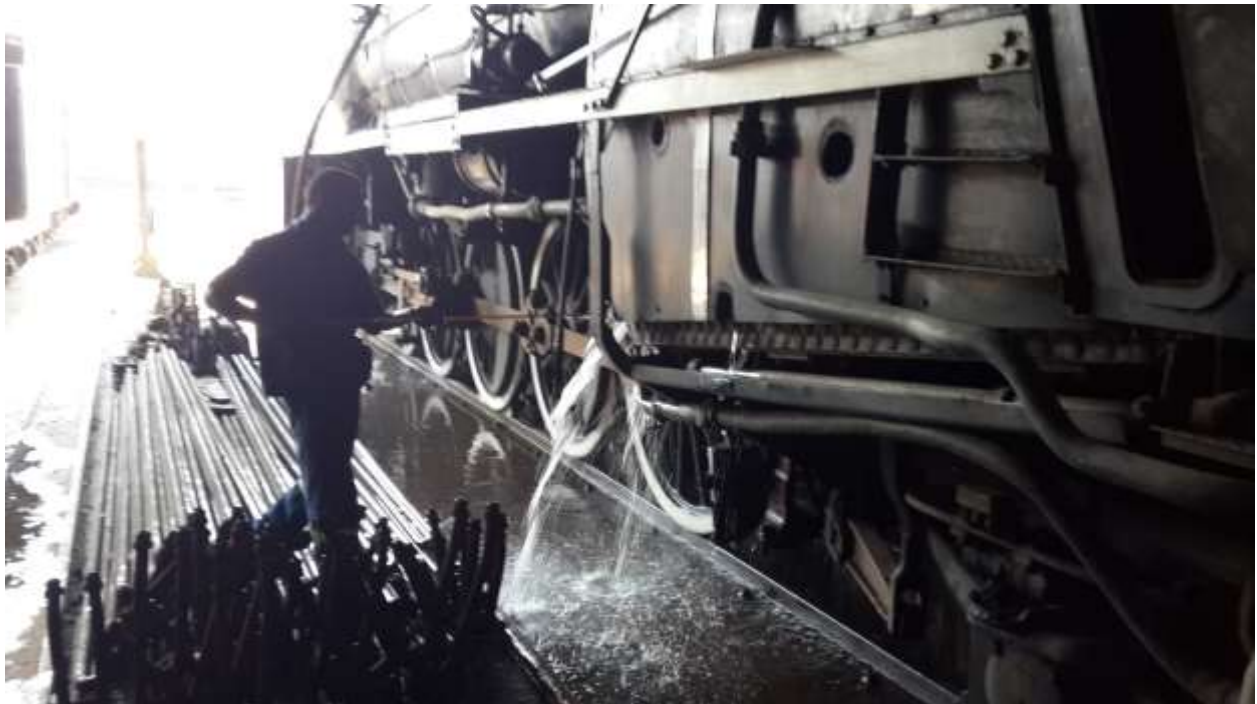
3052 being washed out prior to being re tubed. Picture by FEDRAIL SA
