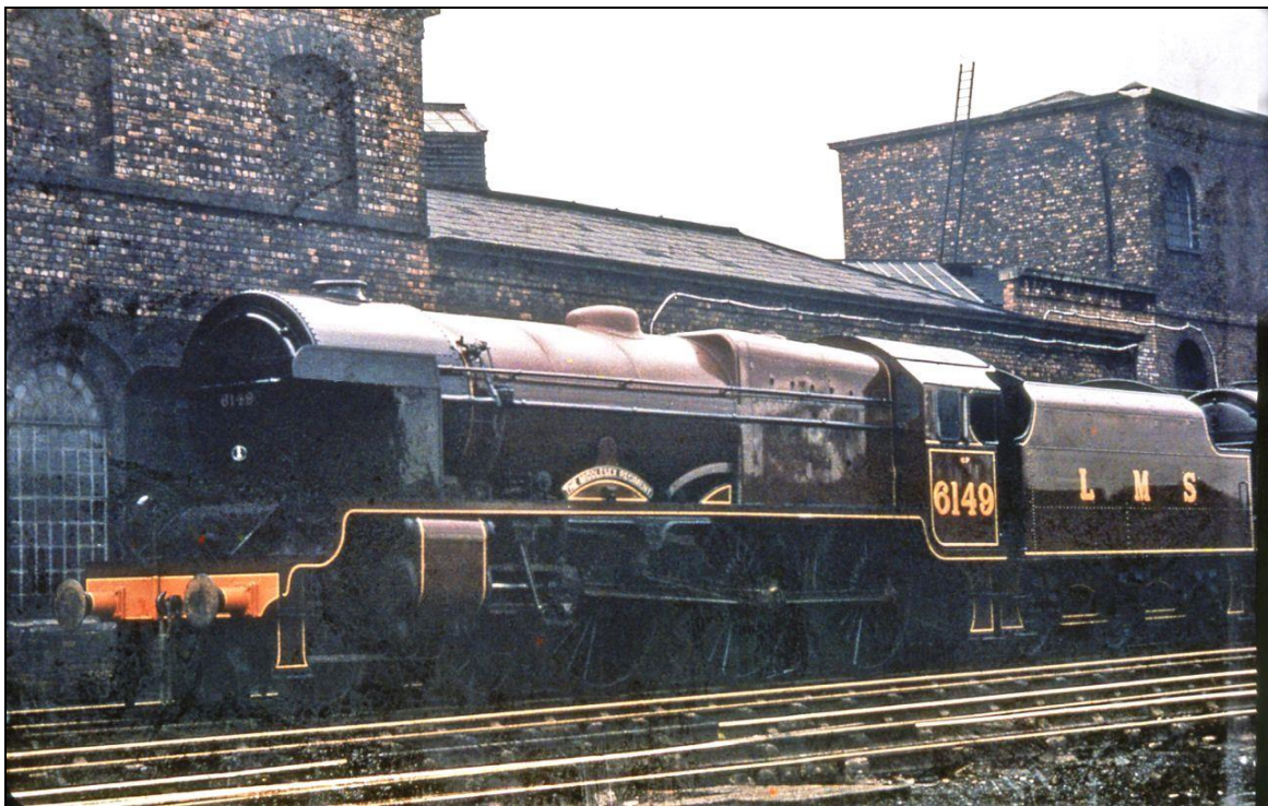
‘Royal Scot’ No 6149 ‘The Middlesex Regiment’ (NB 23644) ex Works at Crewe in April 1937. This locomotive entered service as ‘Lady of the Lake’ and still carries her original NBL parallel boiler.
