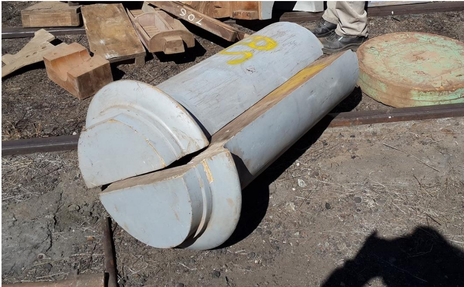
The 6 th class chimney pattern originally from Dunns. Picture by Dave Richardson
