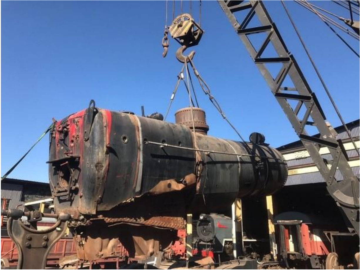
Lifting the boiler from 454.
